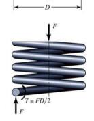
Defining the <u>spring index</u> which is a measure of coil curvature as:
